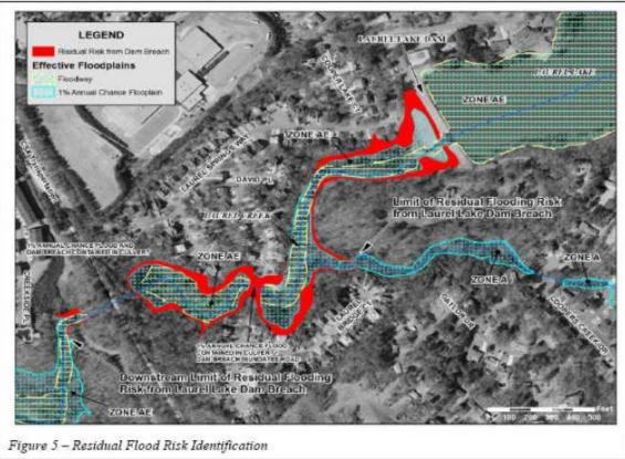
Figures 2-5 are images of enhanced hazard mitigation maps that can be produced via the non regulatory products. The Simplified Dam Break GIS Toolset creates the images that can be leveraged by FEMA for distribution and use by communities.
