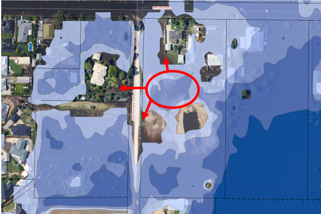
Figure 6: Aerial Photo overlapping with 100 years ARI mapping shows illegal filling on properties and the impact of reduced flood storage in the adjacent areas and properties.
