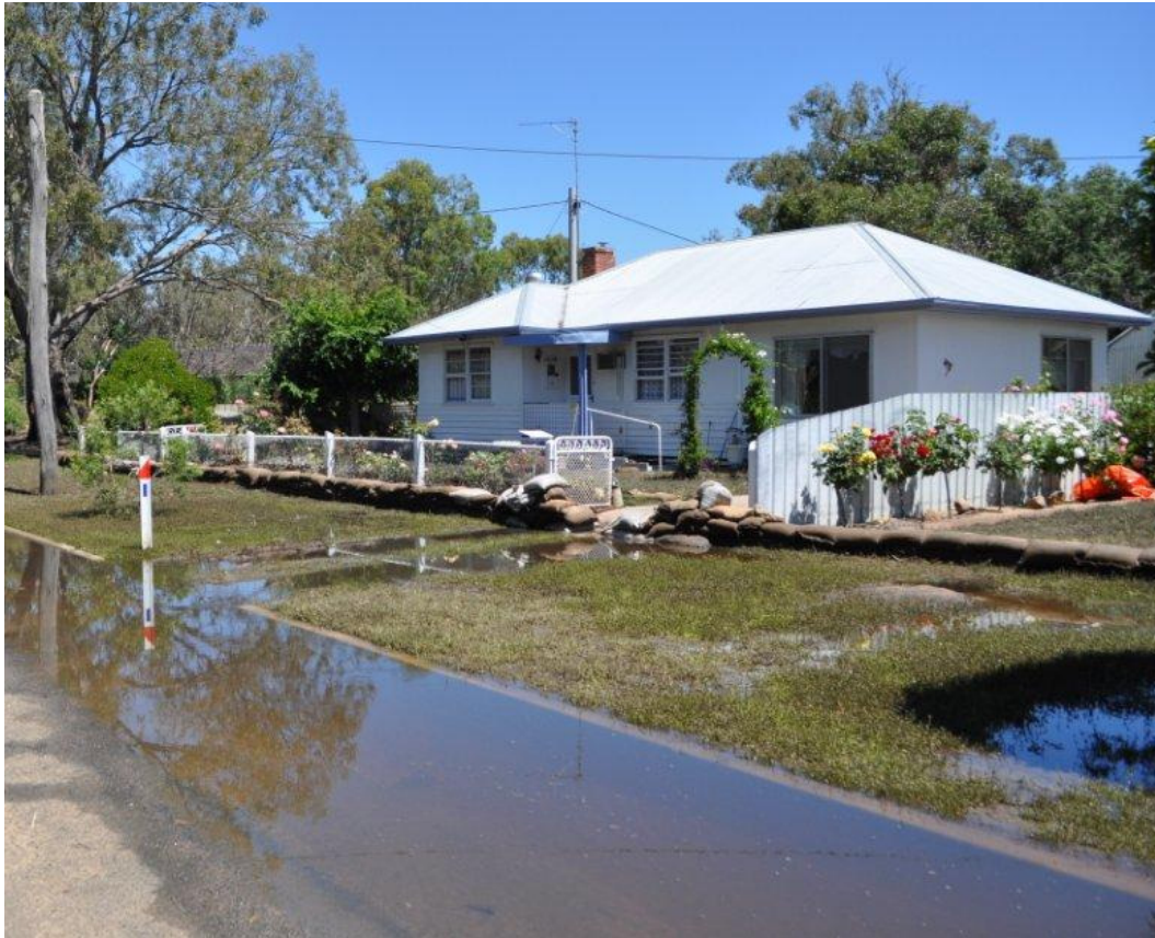
Figure 10: Sandbagging property boundaries instead of houses such as this one in Dimboola was common and reduced overall floodplain capacity.
