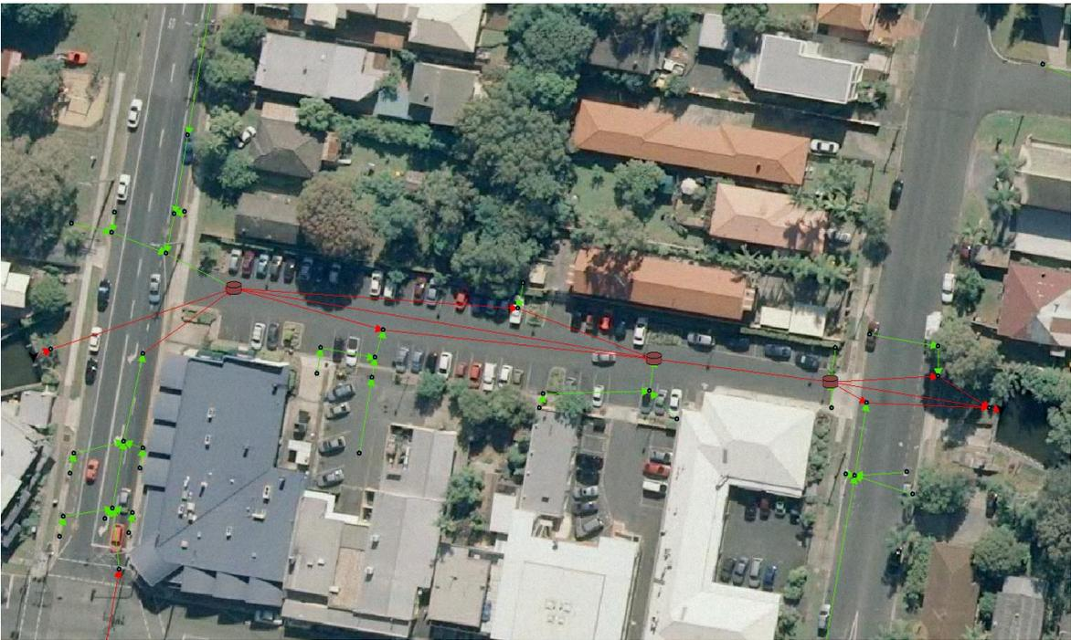
**Figure 4 The resulting geometric network with basins at large structure locations.**
