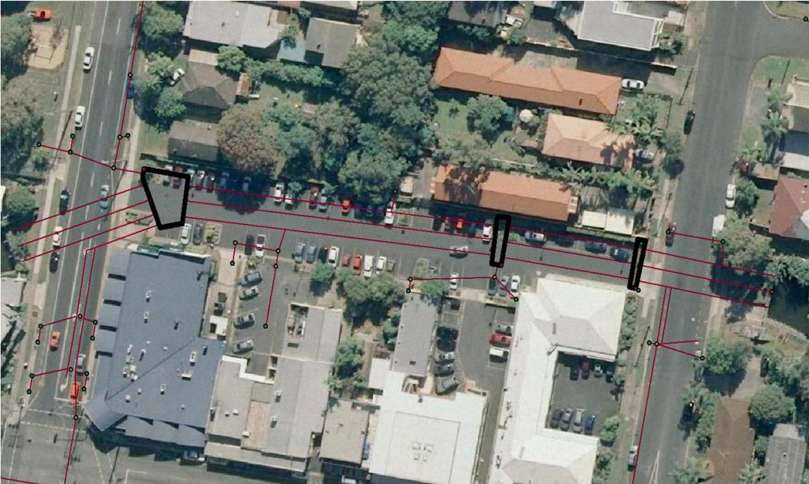
**Figure 3 Polygons boundaries converted to points with 0.1m spacing. Pipes can be snapped to these points using a 0.1m snapping tolerance.**
