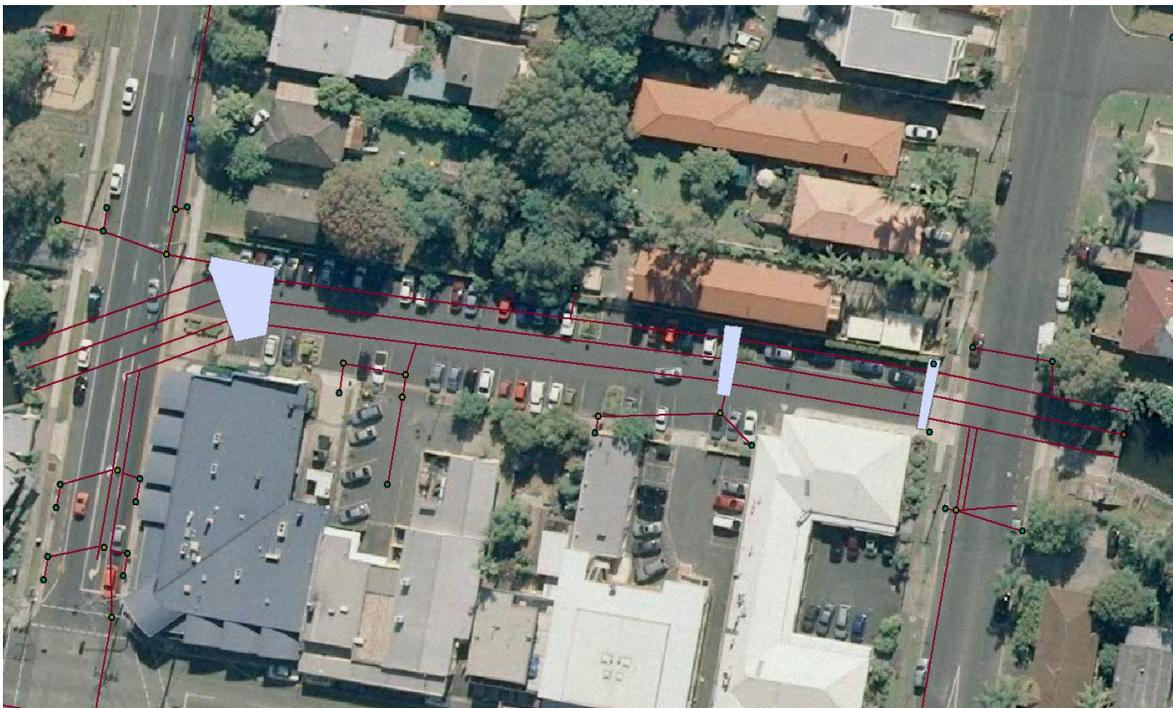
**Figure 2 Raw GIS data with large chambers stored as polygons**
